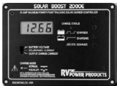
The SolarBoost 2000e was one of the first MPPT charge controller designed specifically for RV use.
