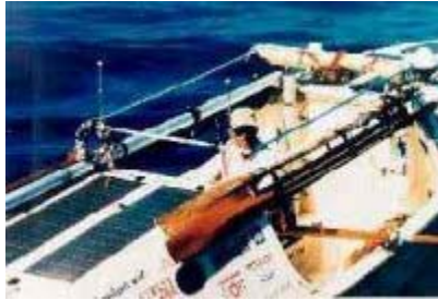
Unisolar solar panels used on back of a boat.
